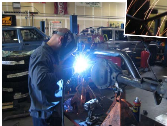
The rear axle truss being welded onto the Dana 44.
