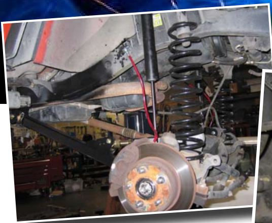
Front suspension done. Note the distinctive square long arms, a Clayton signature.
